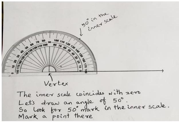
Step 5: Move along that scale and mark a point at the required number of degrees.
