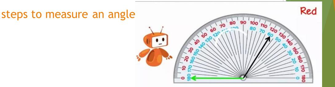
Step 1: place the centre of the proctractor on the vertex of the angle and adjust the protractor so that the base line of the proctor falls along one arm of the angle.
