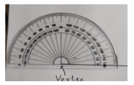
Step 2: Place the centre of the proctractor on the end point of the ray (vertex).
