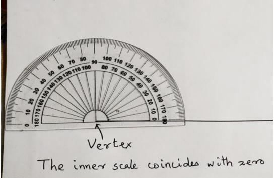
Step 4: Look at the scale which reads zero along the ray which coincides with the base line.
